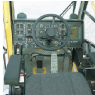
The PAT iFlex 5 graphic display LMI includes a work area definition system which allows the operator to define a preferred working area.
