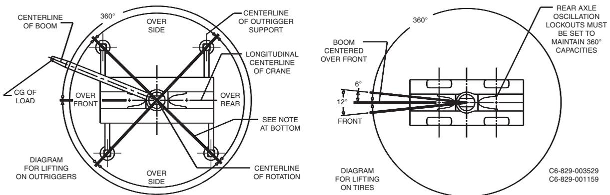
**Bold lines determine the limiting position of any load for operation within working areas indicated.**
