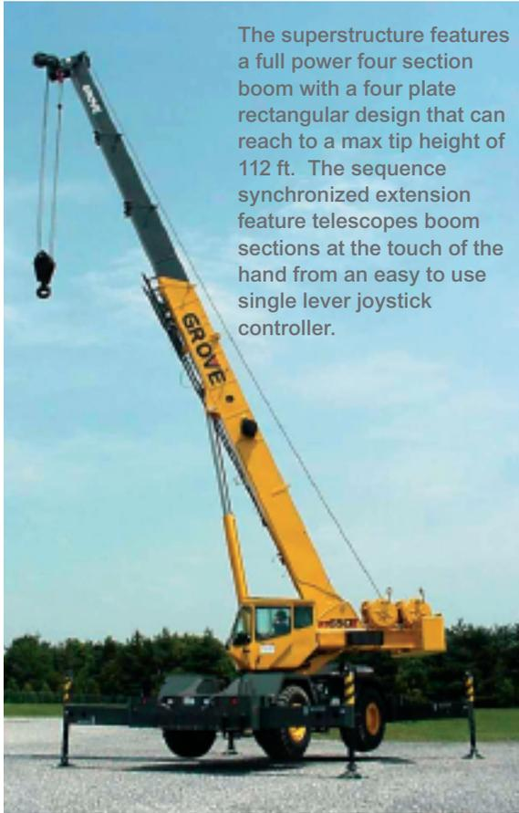
The superstructure features a full power four section boom with a four plate rectangular design that can reach to a max tip height of 112 ft. The sequence synchronized extension feature telescopes boom sections at the touch of the hand from an easy to use single lever joystick controller.
