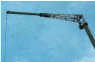
A telescopic swingaway lattice extension easily stows on the side of the base boom for easy transport. With a range of 29-51 ft. the max tip height reaches 162 ft. with a capacity of 6,000 lbs. An optional fixed lattice is also available, reaching a max height of 141 ft.
