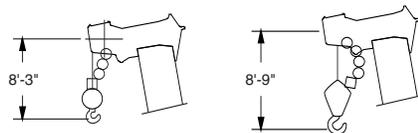
Dimensions are for Largest Grove furnished Hook Block and Headache Ball, with Anti-Two Block Activated.
